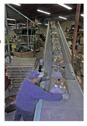
The remaining metal components include the housing supports, metal trays, circuit boards and wires. These are run through the shredder in one batch and are mechanically separated into ferrous and nonferrous metals and low grade circuit boards.
