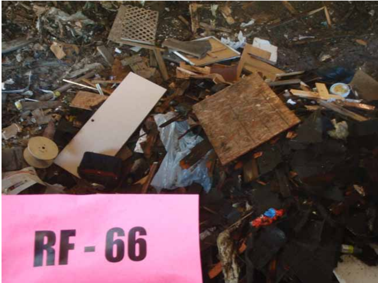
Figure H-11. Clean Engineered Wood and Composition Roofing in Transfer Station Disposed Sample Number RF-66
