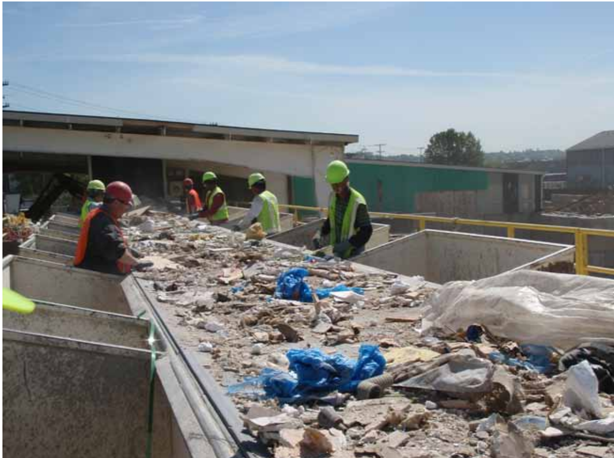
Figure H-12. The End of a Processing Facility Sorting Line
