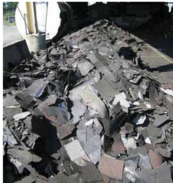
From roof to road - these asphalt shingles will be recycled into new pavement.
