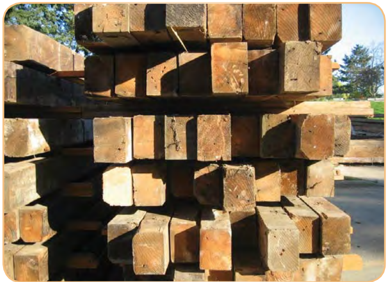
Wood beams from a deconstruction site are salvaged for use in new building construction
