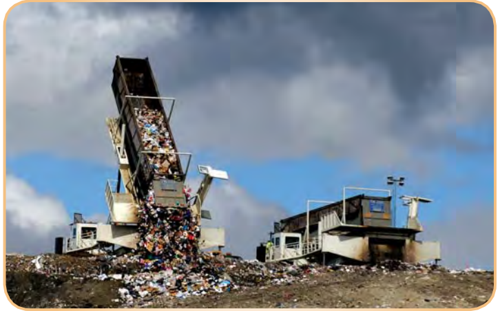
Side-by-side tippers greatly reduce the time required for unloading garbage trailers at the landfill.
