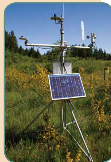
Powered by solar panels, weather stations provide environmental monitoring data at several division facilities.
