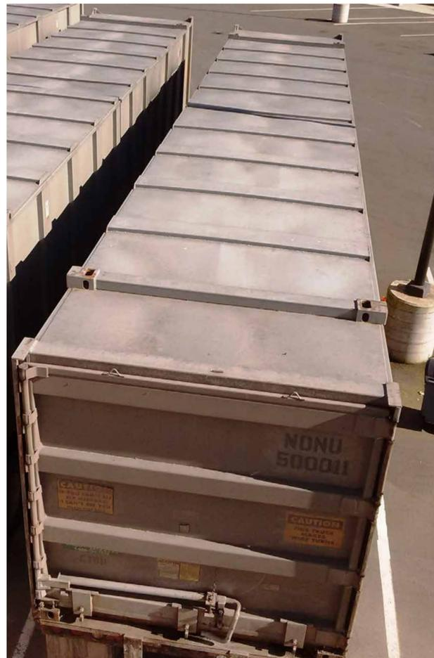
*Compacted solid waste is transported in sealed trailers which help control odor and litter*
