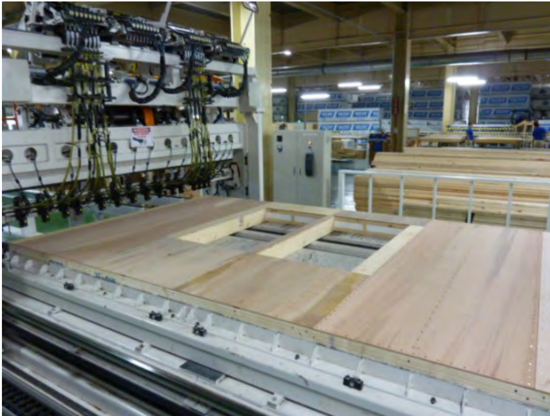
Prebuilt wall panels being fabricated
