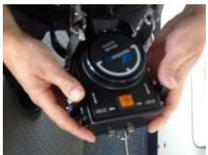
Captain utilizes both thumbs (one for each throttle) as well as center dial when operating the vessel via remote control when docking
