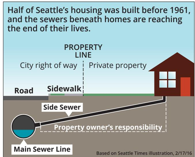
**Figure 3. Seattle faces rising number of side-sewer failures**
