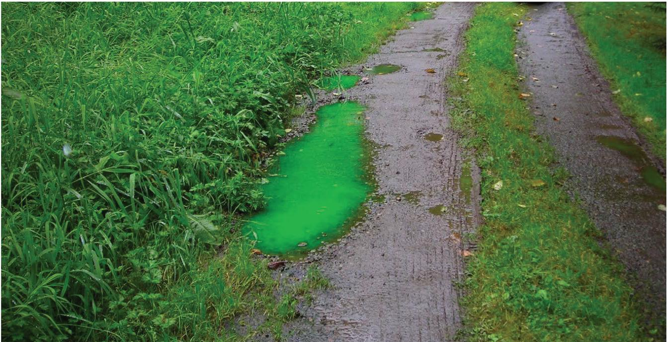
A failure can be confirmed with a fluorescent dye test.
