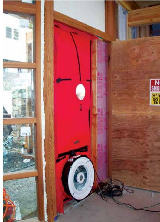
A blower door test during construction measures the home's air leakage at a standardized pressure. Source: O'Brien & Company
