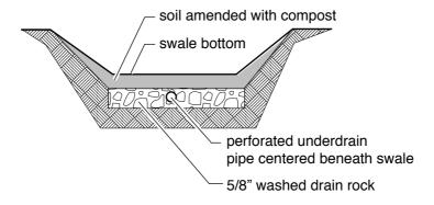
**NOTE:** Underdrain must infiltrate or drain freely to an acceptable discharge point.
