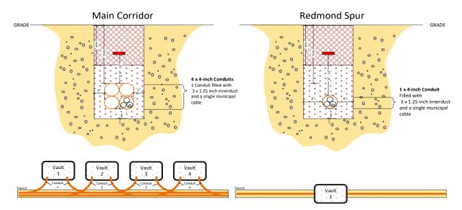
(This is the spec for the existing conduit in RCC Phase 1 and 2)
