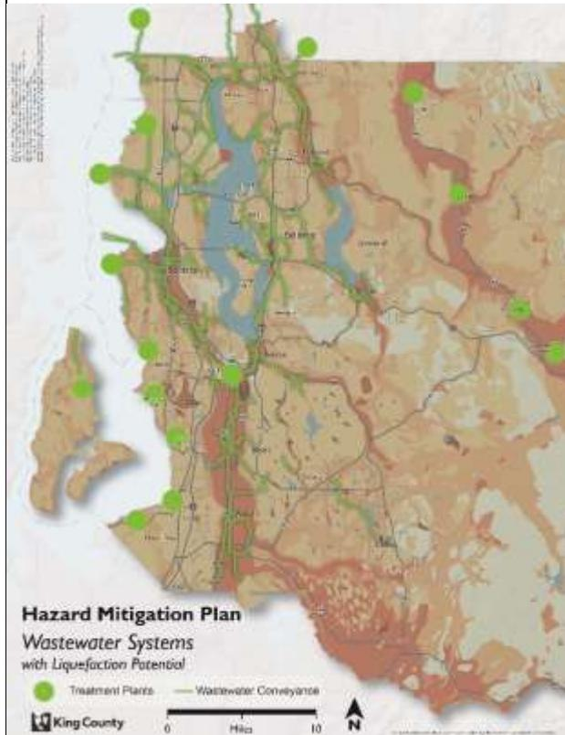
Water/Wastewater: Water and wastewater systems are among the most vulnerable to an earthquake of all lifeline infrastructure. Pipelines, especially those over NEHRP class D, E, and F soils, are vulnerable to rupture. King County maintains a wastewater treatment system that is connected to dozens of smaller systems and operates multiple water treatment plants. There are also many separate water systems that operate their own conveyance systems and reservoirs.
