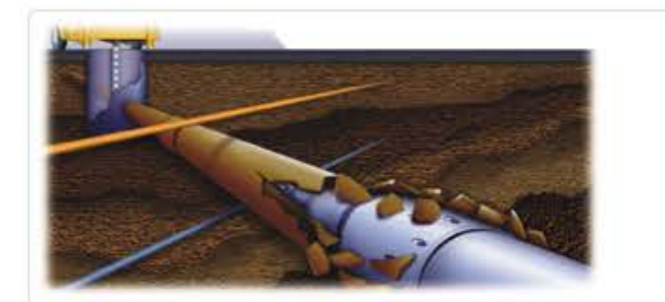
A pipe cutter breaks up an existing pipe before pulling in a new pipe.
