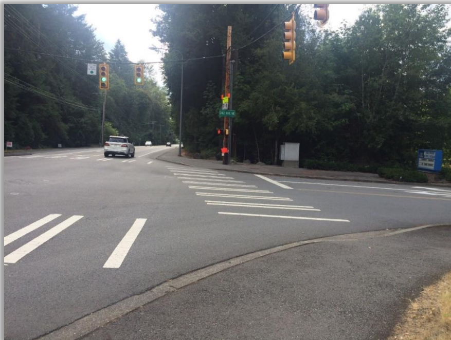
30. Looking west on northeast corner of NE 8 th Street and 242 nd Avenue NE. Conditions: 45 feet roadway across Inglewood Middle School entrance, 6 feet asphalt sidewalk, 4 feet paved shoulder, signalized intersection.
