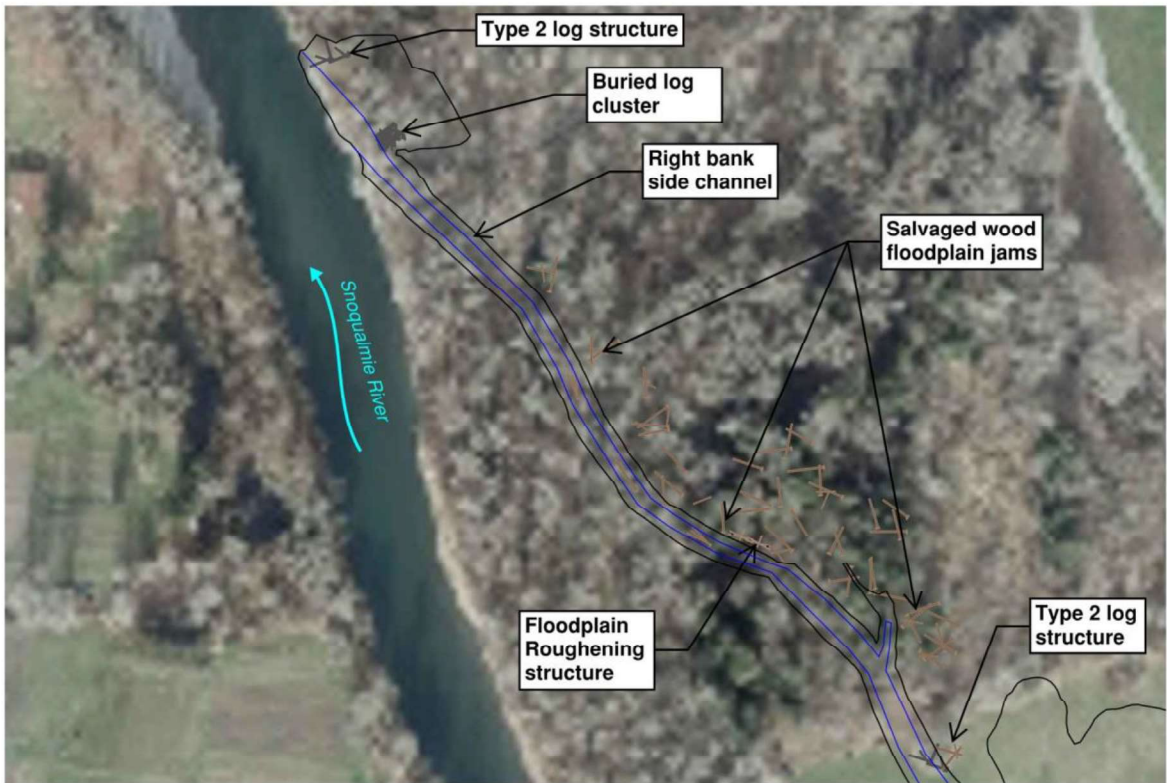
Figure 13 – Placement of floodplain roughening ELSs and salvaged wood floodplain jams and individual logs in the right bank floodplain adjacent to the constructed right bank side channel.
