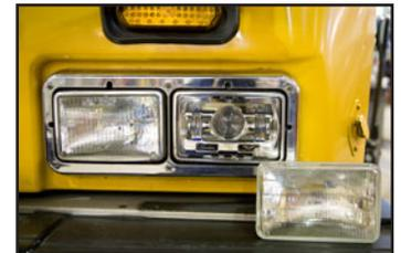
**A new LED low-beam lamp (mounted in bus, on right) installed next to a regular high-beam lamp.**
