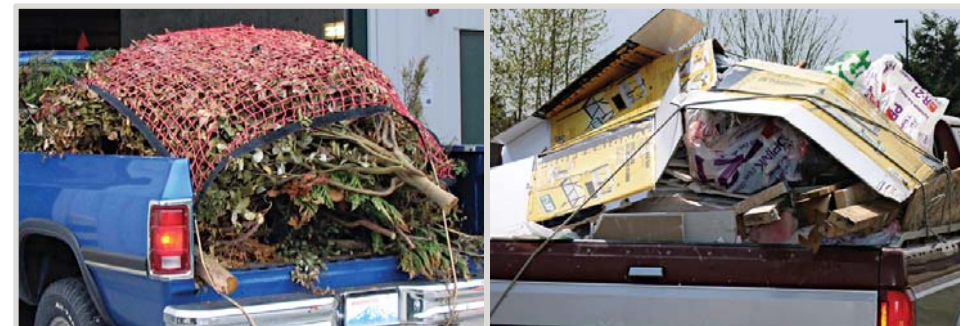
These loads are not secure! The rope and netting as attached are not adequate to ensure that nothing can leave the vehicle while it is moving.
