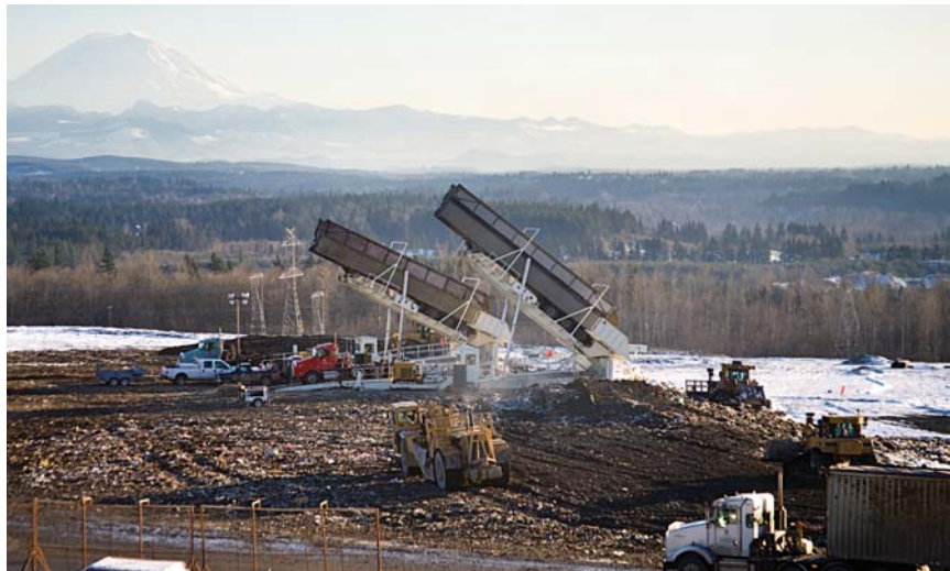
Side-by-side tippers keep greatly reduce unloading time for solid waste transfer trailers.
