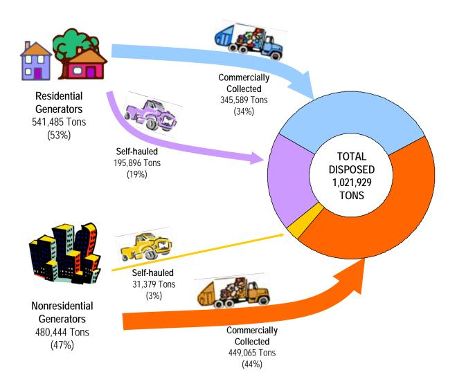
Figure 1-1. Waste Substreams & Tonnages in 2007
