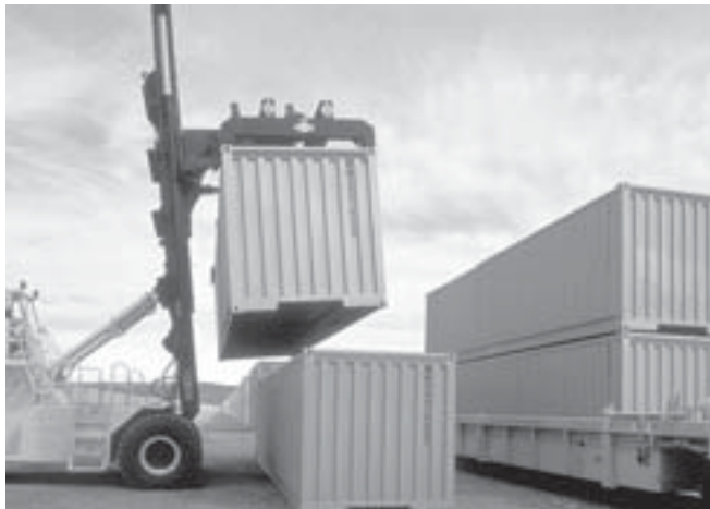
▲ Containers full of MMSW from the City of Seattle are hoisted onto a train for export to a landfill in Oregon
