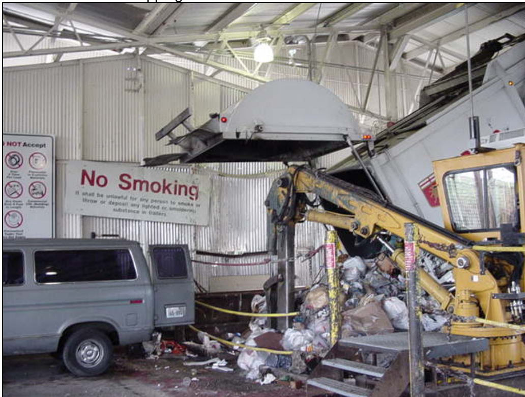
The back door of a commercial vehicle opens over a self-haul vehicle while dumping garbage into the same chute.
