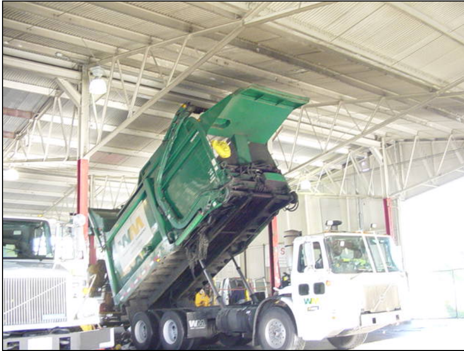
A commercial garbage truck with trailer raised inches from the roof.
