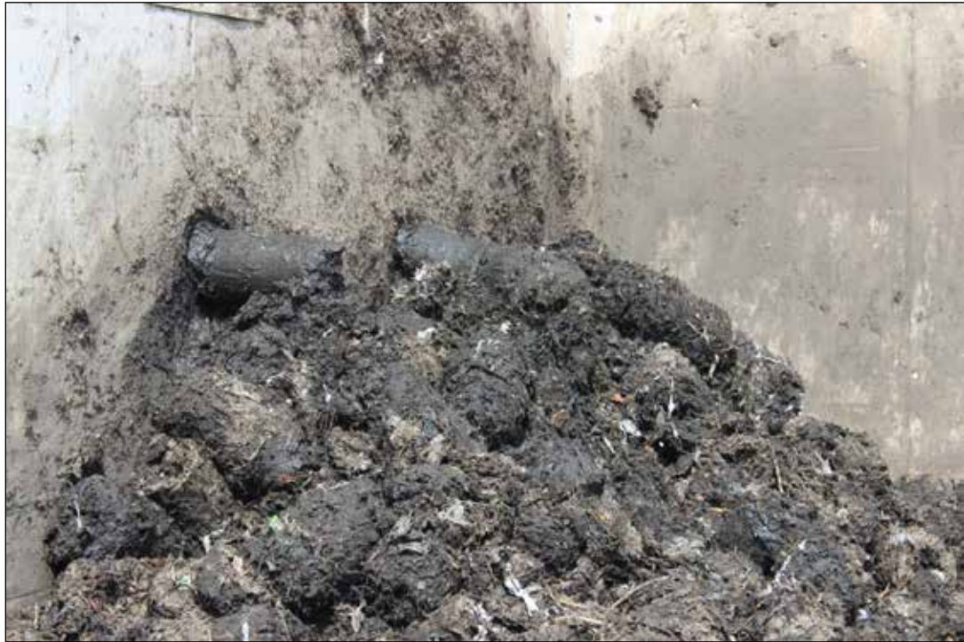
Figure 3-6. FITEC, Rothmuhle Biogas Plant: Extruded Solid Fraction from Biosqueeze Unit
