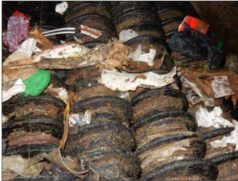
Figure 3-2. Mechanical Sorting - Disc Screen of Organics Feedstock
