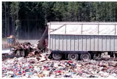
In the mid-1980s, walking floor trailers replace "slam dunk" trailers, allowing multiple loads to be dumped simultaneously.
