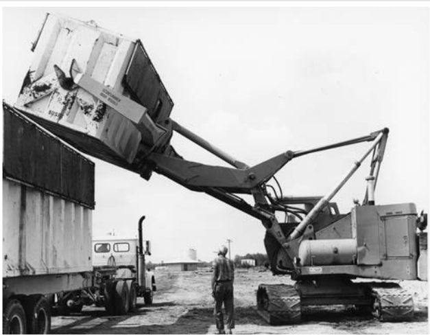
"Slam dunk" trailers are used to transport solid waste from King County transfer stations to Cedar Hills.
