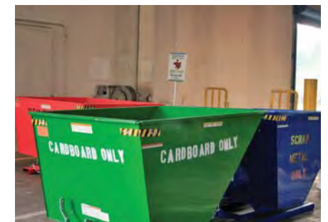
Receptacles are color-coded – green for cardboard, blue for scrap metal, and orange for clean wood – so customers can sort recyclable materials instead of dumping them directly onto the tipping floor.
