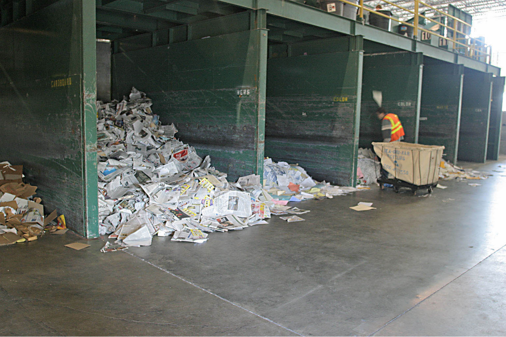
As the staff sort the paper, it falls into separate compartments underneath the sorting line.
