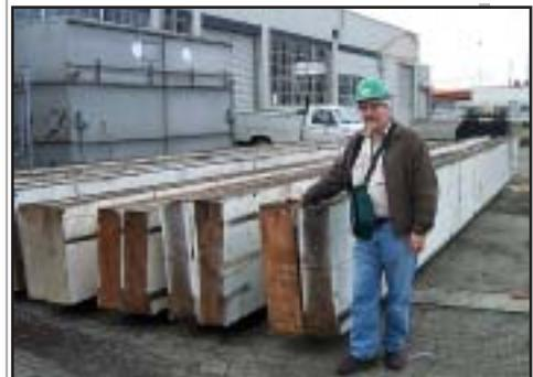
*60 foot long old growth timber beams ready for shipping and minor re-milling.*
