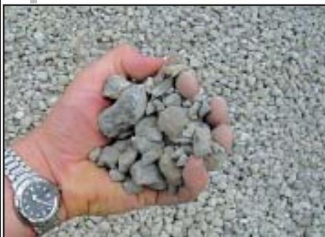
"The Nibbler" and a concrete crusher reduced concrete blocks into 1-inch diameter concrete pieces.
