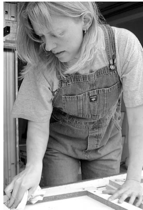
Ameé Quiriconi oils a mold before pouring a Squak Mountain Stone tile, a new product that uses about 65 percent recycled material.
