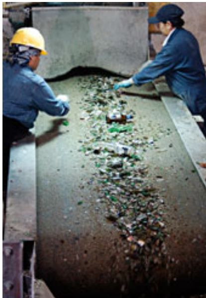
Sorting glass at Fibres International recycling facility in Seattle.
