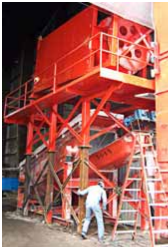
Machine designed by Recovery 1 to crush gypsum for recycling.
