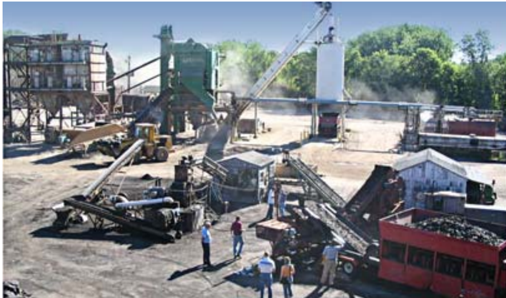
Omann Brothers Inc. asphalt shingle recycling and hot-mix asphalt plant near St. Michael, Minnesota.
