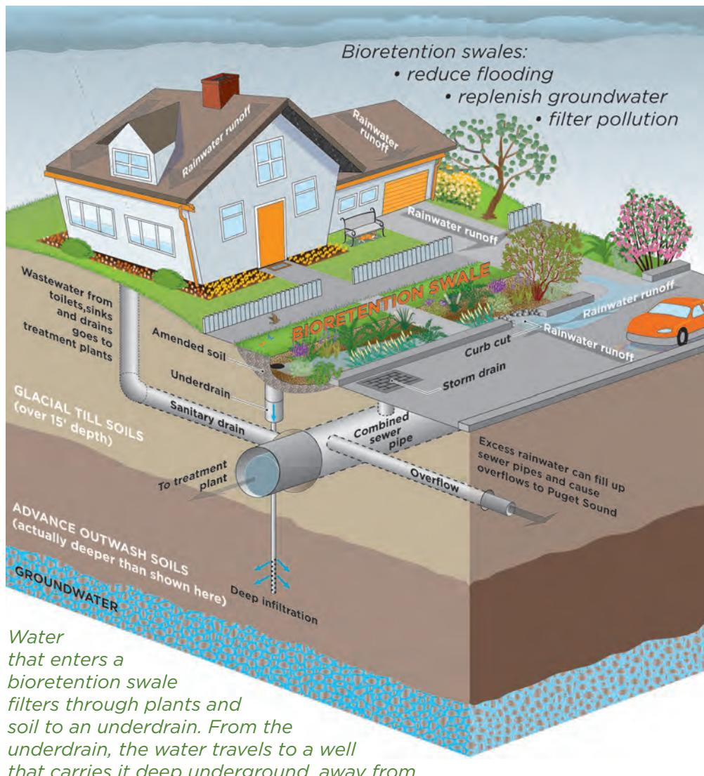
*Bioretention swales help control sewer overflows and prevent polluted rainwater from entering Puget Sound—the number one source of pollution to Puget Sound.*
