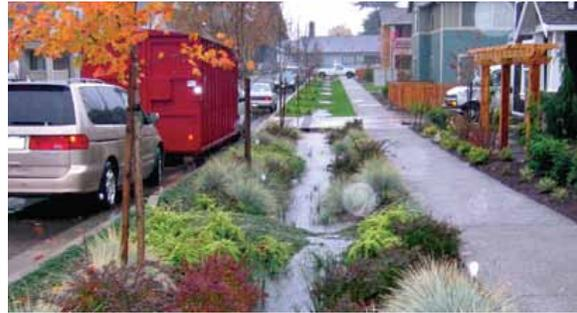
*After a big rain, wetlands and bioswales clean the water and allow it to soak into the ground over several hours.*
