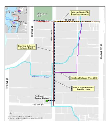
In the summer of 2011, KLB Construction, supervised by King County construction managers, will begin installing a new, larger sewer pipe along Southeast 3rd Street and 102nd Avenue Southeast to replace the existing city and county pipes.
