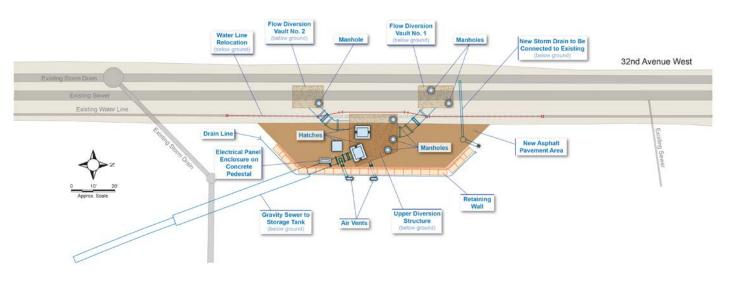
On the east side of 32<sup>nd</sup> Avenue West, a pullout will allow crews access to above ground equipment in a vault. A permanent retaining wall will be installed behind the pullout. Affected areas of pavement will be restored, and catch basins will be added in the project area to help manage stormwater.
