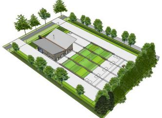
The current project rendering depicts the vegetative buffers that will be used to screen and soften the appearance of the site. In addition, the team removed a sidewalk in front of the building and replaced it with vegetation to reduce pavement in an area where it was feasible to do so.
