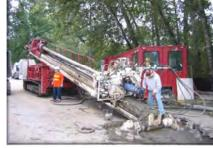
Horizontal Directional Drilling (HDD) Rig used for **Drilling and Reaming**
