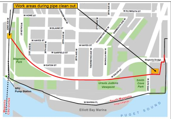
Crews will clean out the damaged pipe from the Magnolia Wet Weather Storage facility near Smith Cove and from an underground diversion structure near 32nd Ave. W.
