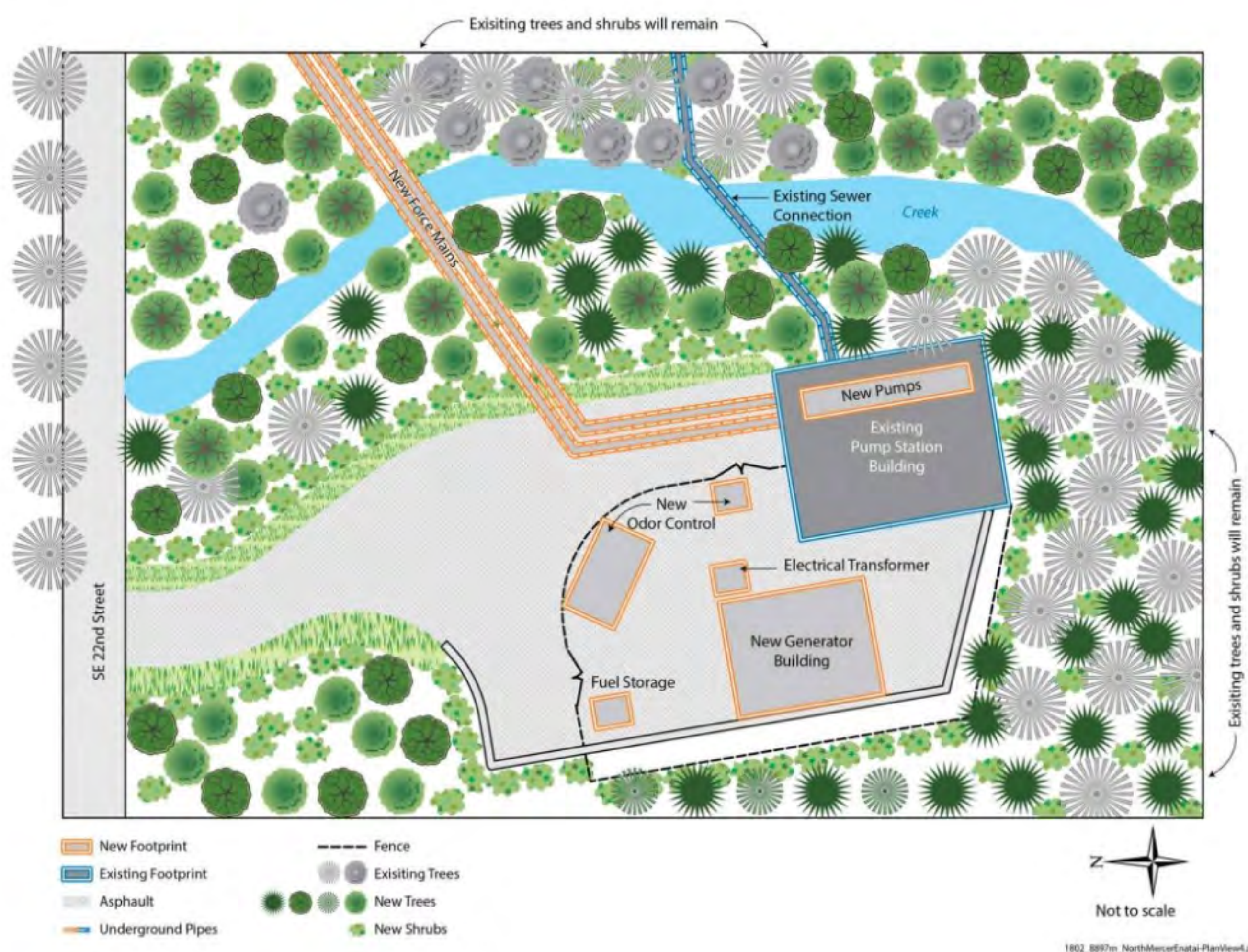
Conceptual schematic plan for North Mercer Pump Station
