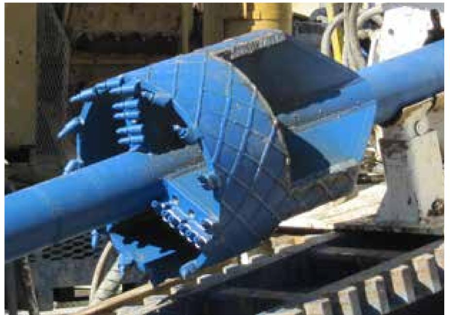
Crews install the new pipeline using special equipment that drills a small hole along the future pipe route. There is a wire on the surface that tracks the location of the drilling equipment underground (above, left). Crews enlarge the hole using equipment called reamers (above, right) until it is large enough for the new pipe. A special type of mud is used to keep the hole open until the pipe is pulled into place.
