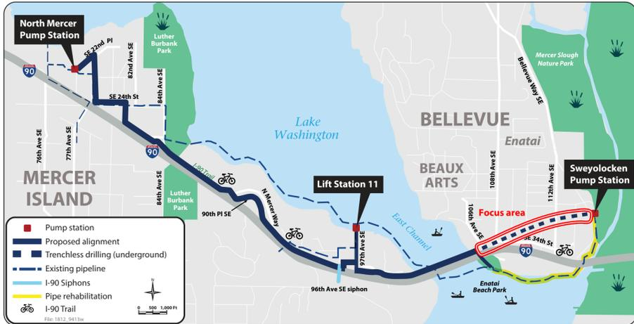
In order to increase capacity in our sewer pipes, this project includes the installation of a new sewer pipe under the Enatai hillside from Enatai Beach Park to the Sweyolocken Pump Station.
