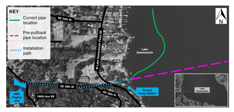
King County has worked to minimize pullback impacts by staging the pipe on Lake Sammamish and fusing all pieces together in advance. A few days before installation, crews will straighten out the pipe on the lake to prepare it for the pull.
