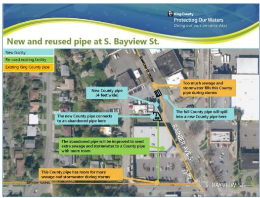
Figure 13. Rainier Valley Wet Weather Storage Project New and Reused Pipe
