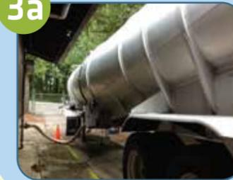
A small amount of solid material is periodically removed from the bottom of the clarifier to prevent buildup. This excess waste is loaded into tanker trucks and taken to South Treatment Plant in Renton for recycling.
