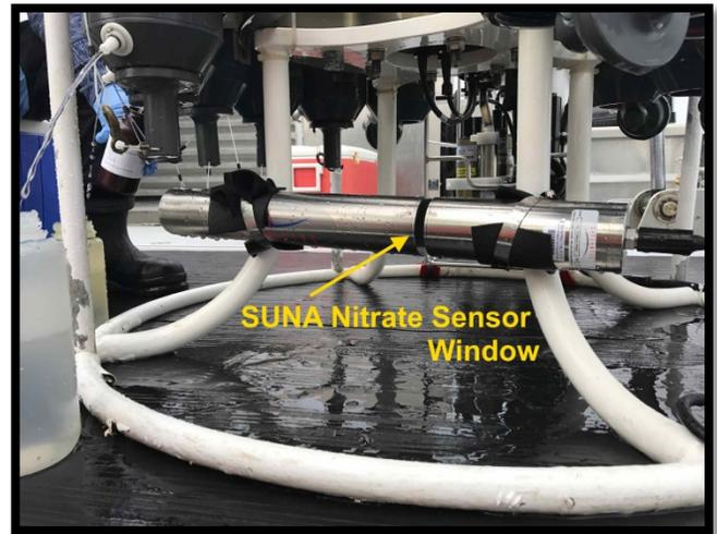
**Figure 6.** Washington State Dept. of Ecology's Submersible Ultraviolet Nitrate Analyzer (SUNA) pictured above attached to King County's water sample carousel frame. This new instrument rapidly measures changes in nitrate as the carousel is lowered through the water, and was recently added to provide more information on nutrient dynamics.
