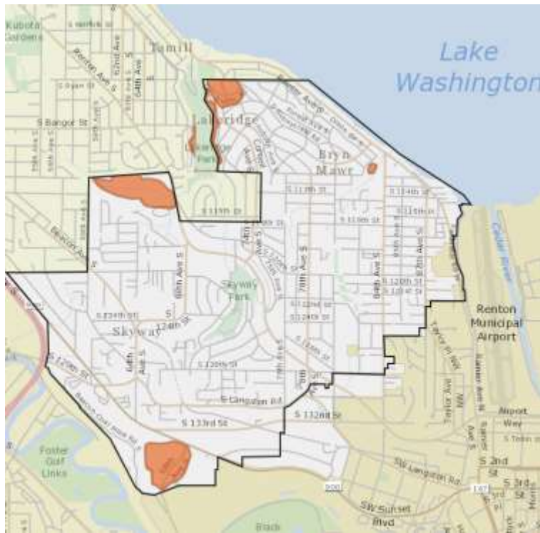
Figure 7: Potential Landslide Hazard Areas (Plus 50-Foot Barrier) in and Around Skyway Water and Sewer District (in orange)
