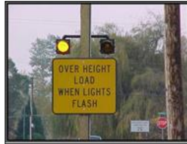
Over height warning systems have sensors that activate warnings signs when a vehicle is taller than allowed.
