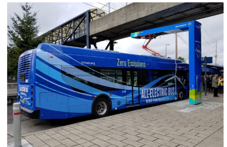
A battery-electric bus in Portland is charging at a transit center bus stop. The pantograph is lowered and in contact with rails on the roof of the bus.
