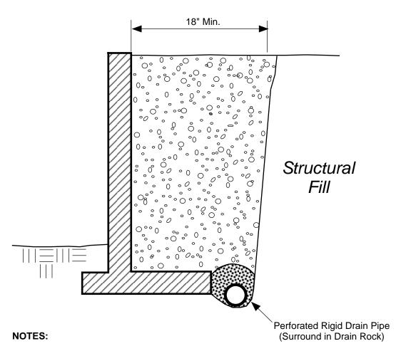
Free-draining Backfill should consist of soil having less than 5 percent fines.
