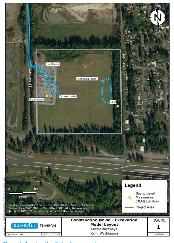
**Figure 1. Construction Noise Assessment**
