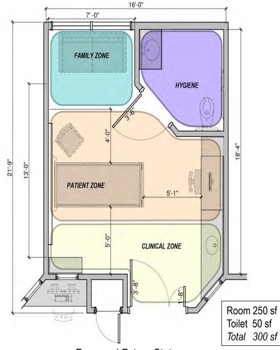
Bed clearance in the existing space is close to meeting FGI requirements for Intermediate Care beds, but the toilet rooms would need to be renovated to add a hand wash sink and provide appropriate space around the toilet.
